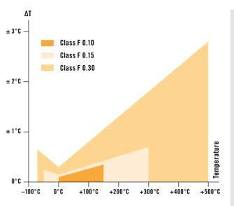
Tolerances of base values for Pt temperature sensors are specified in DIN EN 60751.
