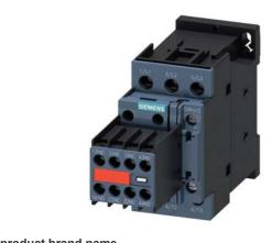
Power contactor, AC-3 25 A, 11 kW / 400 V 2 NO + 2 NC, 230 V AC, 50 / 60 Hz, 3-pole, Size S0, Screw terminal Captive auxiliary switch
