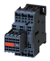
Power contactor, AC-3 25 A, 11 kW / 400 V 2 NO + 2 NC, 110 V AC, 50 Hz, 120 V, 60 Hz, 3-pole, Size S0, Spring type terminal Captive auxiliary switch
