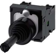
Coordinate switch, 22 mm, round, plastic, black, 2 switch positions, vertical, momentary contact type, without mechanical interlocking in O position, with holder, 1 NO, 1 NO, screw terminal, with laser labeling, upper case and lower case, always upper case at beginning of line
