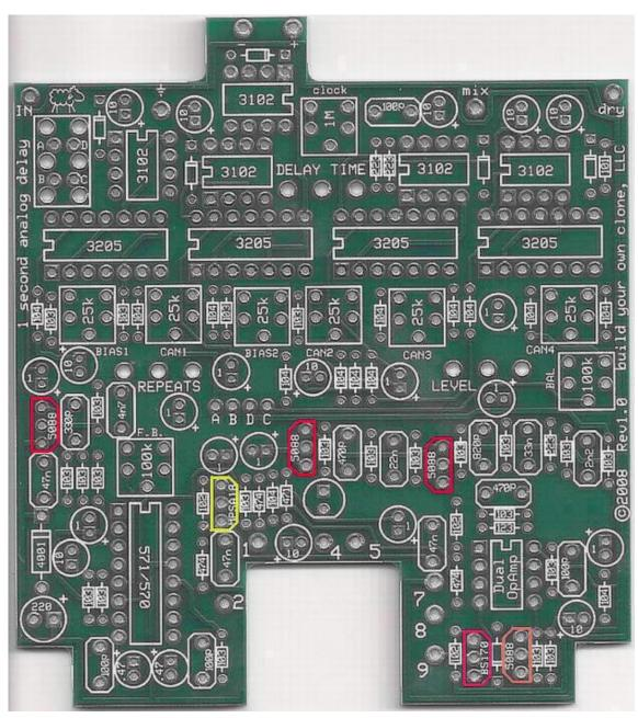
STEP 4: Add the transistors. Match the flat side of the transistor to the flat side of the layout on the PCB. One MPSA18 goes in the space highlighted in yellow. One BS170 goes in the space highlighted in pink. One 2N5088 goes in the space highlighted in orange. And remember that three MPS6521 transistors go in the spaces highlighted in red even though the PCB calls for 2N5088. If you have a Rev1.1 PCB or higher, the parts numbers of the transistors will be labelled correctly.
