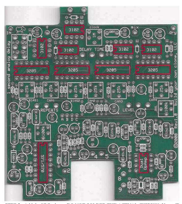
STEP 2: Add the IC Sockets. DO NOT SOLDER THE ACTUAL CHIPS!!!! You will put the chips into the sockets in the "Installing the ICs" portion of the instructions. See page 22 - 23 for more details. Each socket has a notch in one end. You should match that notch up with the layout on the PCB and solder the socket directly to the PCB.
