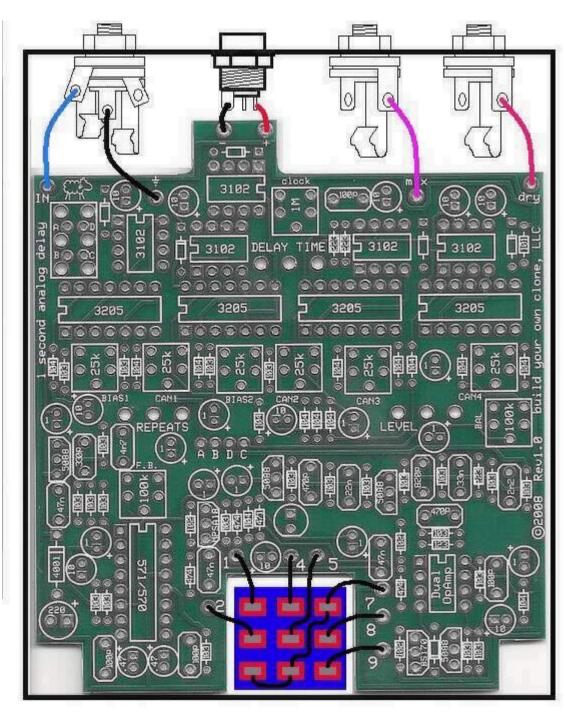
Step 4: Wire the "ABCD" jumpers. Use 4 pieces of wire approx. 3" long. You are simply connecting the "A" eyelet next to the toggle switch with the "A" eyelet more towards the center of the PCB. And "B" to "B", "C" to "C", and "D" to "D". Wire the C and D eyelets first. Then wire the A and B eyelets.
