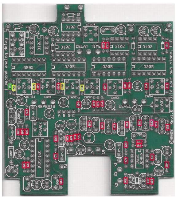
Add the resistors. Remember that the four 10k resistors highlighted in yellow should actually be 1k, the 100k highlighted in green should actually be 10k, and the 22k highlighted in pink should atually be 15k. If you have a Rev1.1 PCB or higher, the resistor spaces will be labelled correctly. A space for the 33k resistor has been added to the PCB and should be soldered at this time.
