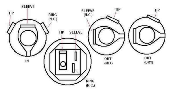
Step 1: Install the 1/4" jacks to the enclosure. Be sure to turn the OUT jacks 1/4 turn counter clockwise so that their prongs do not short out against the delay time pot.
