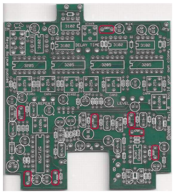
STEP 7: Add the ceramic disc capacitors. These are not polarized and can be inserted into the PCB in either direction.
