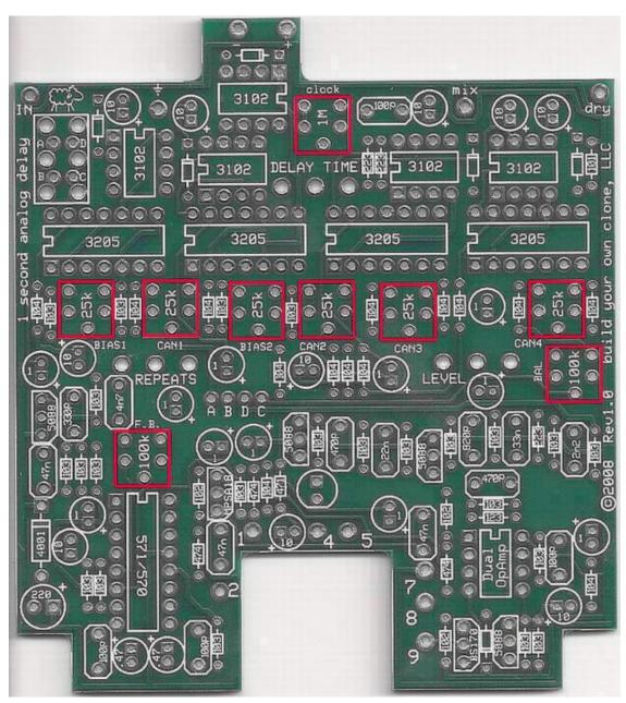
STEP 5: Add the internal trimpots. Many people get confused by these because the trimpot itself only has 3 legs, but the PCB has 5 holes. The PCB has 5 holes so that it can accomodate a variety of different trimpot brands and models. There should only be one way the trimpot will fit into the PCB without having to bend the legs.
