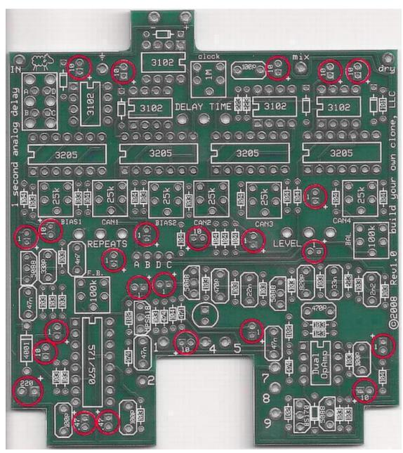
STEP 8: Add the aluminum electrolytic capacitors. These are polarized. The positive end will have a longer lead and should go in the square solder pad. The negative end will have a shorter lead with a black strip running down the body of the capacitor.
