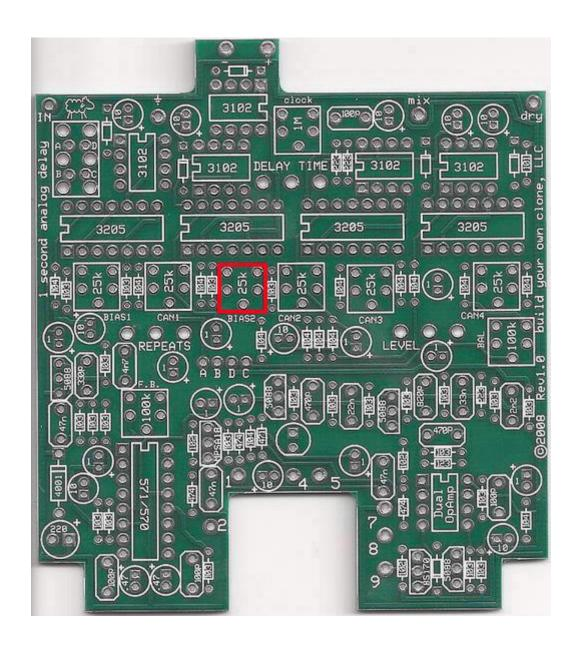
Step 6: Set the BIAS2 trimmer. The first thing you must do is **MAKE SURE THE LONG/SHORT SWITCH IS IN LONG MODE!** Flip the toggle bat so that it is pointing up towards the jacks. You should not hear any echoes again. Now adjusts the BIAS2 trimmer so that you can hear echoes. Now find the "working" range of the trimpot and set it in the middle. Now use your ears to find the best sounding repeats.
