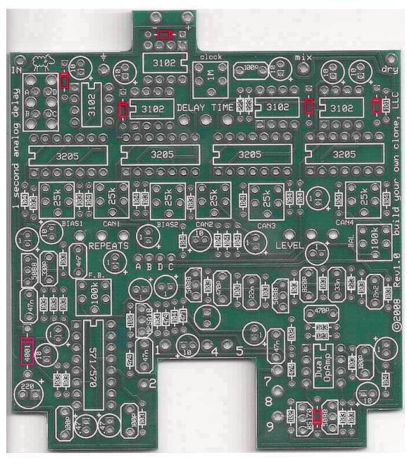
STEP 1: Add the diodes. There are six 1N914 and 1 1N4001 diodes. Be sure to matched the end of the diode with the stripe to the layout on the PCB. The stripped end should go in the square solder pad.
