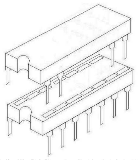
The BBD chips will be slightly different. They will only have 8 pins, but in a 14 pin space. The 6 center pins (3 on each side) of the socket are not used. You may see traces on the PCB, but they are simply being used as vias. So don't let this confuse you. Treat the BBD chips as if they were 14 pin chips and put them in the 14 pin socket.
