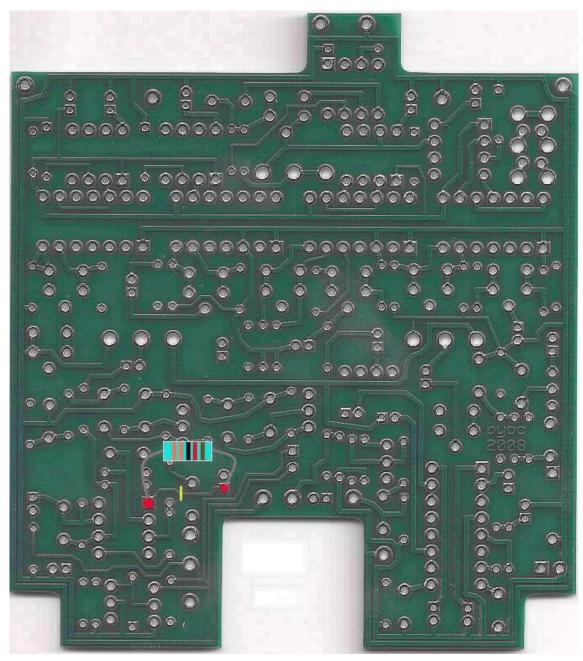
You'll also need to make a minor adjustment to the PCB. You will need to use a utility knife, razor blade, exacto knife or something sharp to cut one of the traces on the bottom side of the PCB. You will make the cut at the yellow line highlighted in the diagram above. You will then need to add a 33k resistor to the bottom side of the PCB, connecting it to the solder pads highlighted in red. You should save this for the step till the end of the "populating the PCB" process. You will be reminded.
