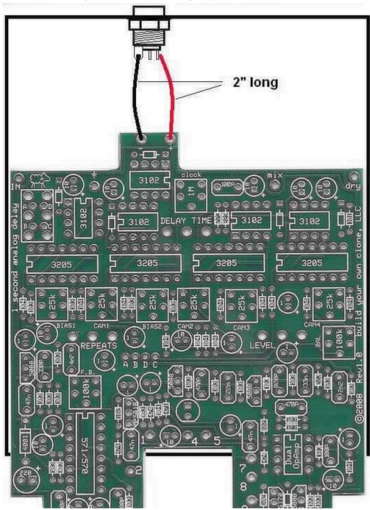
Step 2: Connect the TIP (negative) terminal of the DC adaptor jack to the "-" eyelet on the PCB with 2 inches of hook up wire. Connect the SLEEVE of the DC adaptor jack to the "+" eyelet on the PCB with 2 inches of hook up wire.
