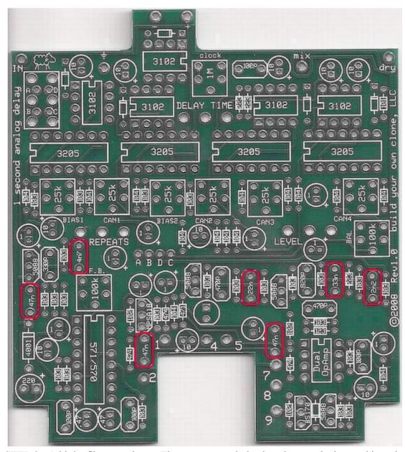
STEP 3: Add the film capacitors. These are not polarized so they can be inserted into the PCB in either direction.
