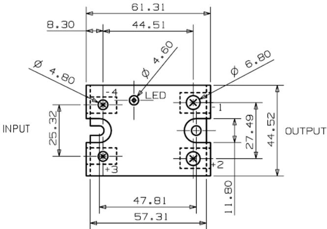
Figure 19: Installing the Solid-state Relay
