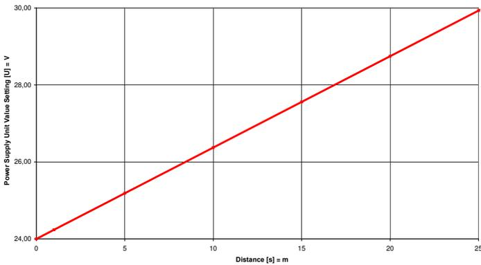
Figure 20: Line Drop,  $1.5mm^2$  Cable Cross-Section
