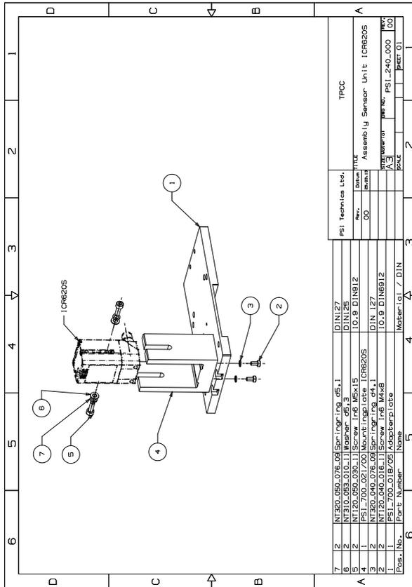
Figure 35: SICK Lector<sup>®</sup>620 Professional / ICR620 Mounting Instructions
