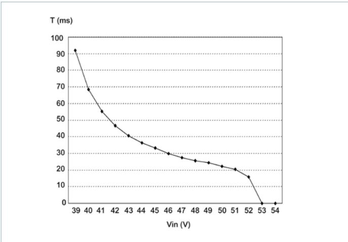
Figure 1 — Shut-down time of M-FIAM5B vs. overvoltage
