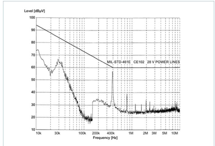
Figure 2 — Conducted noise; M-FIAM5B and Model V24A12M400B DC-DC converter operating at 28V<sub>DC</sub>, 400W
