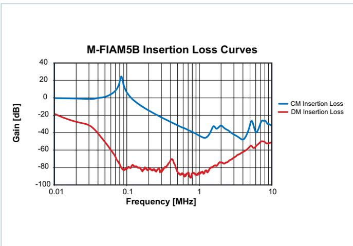
Figure 5 — Insertion loss
