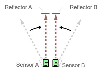
Note: From behind the Sensor Pair, Sensor A may be either to the left or to the right of Sensor B. This will depend on whether the Sensor Pair is mounted on the left or the right of a door. The alignment process will be the same for either position.
