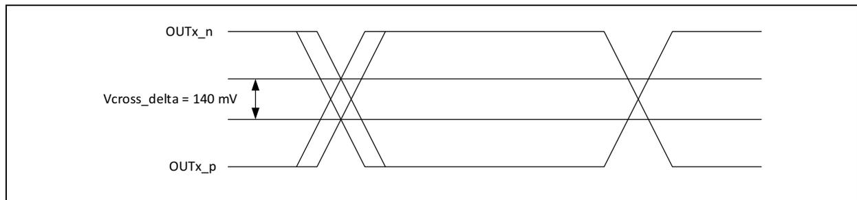
**FIGURE 1-2:** Single-Ended Measurement Points for Delta Cross Point.
