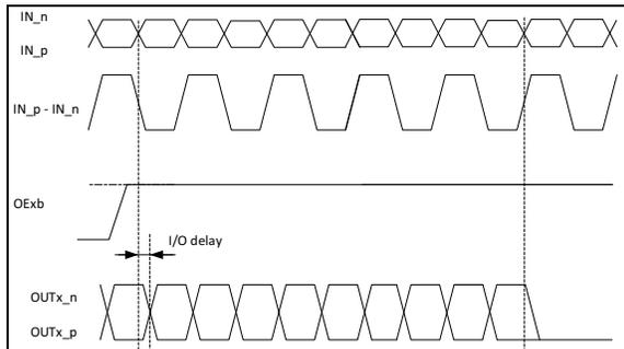
**FIGURE 4-6:** OExb Deassertion (Output Disable) Timing Diagram.
