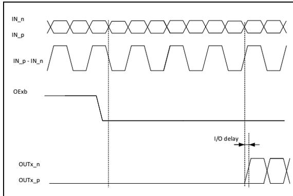
**FIGURE 4-5:** OExb Assertion (Output Enable) Timing Diagram.
