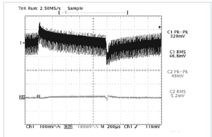
**Figure 24** — V300B12C250B and μRAM; Input and output dynamic response  $C_{TRAN} = 820\mu F$  Electrolytic; 30% of load step of 6A (10A – 16A);  $R_{HR} = 80k\Omega$  (configured as in Figure 8 w/o Trim)
