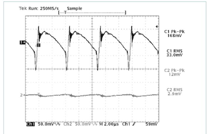
**Figure 22** — V375B12C250B and μRAM; Input and output ripple @50% (10A) load CH1 =  $V_{IN}$ ; CH2 =  $V_{OUT}$ ;  $V_{IN} - V_{OUT} = 305mV$ ;  $R_{HR} = 80k\Omega$  (configured as in Figure 7 w/o Trim)
