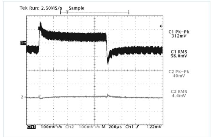
**Figure 20** — V375A28C600B and μRAM; Input and output dynamic response no added  $C_{TRAN}$ ; 20% of 20A rating load step of 4A (10A – 14A);  $R_{HR} = 178k\Omega$  (configured as in Figure 7 w/o Trim)
