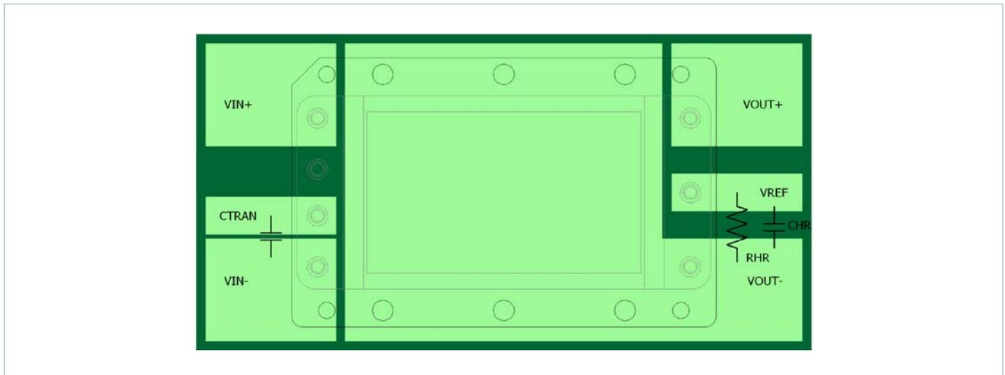
Figure 18 — Recommended copper patterns, top view
