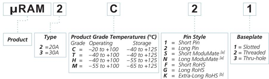
[a] Compatible with the ModuMate interconnect system for socketing and surface mounting
