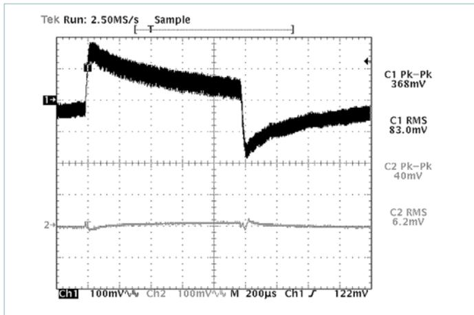
**Figure 21** — V375A28C600B and μRAM; Input and output dynamic response  $C_{TRAN} = 820\mu F$  Electrolytic; 32.5% of load step of 6.5A (10A – 16.5A);  $R_{HR} = 178k\Omega$  (configured as in Figure 7 w/o Trim)
