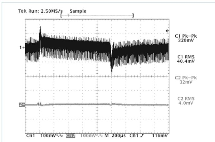
**Figure 23** — V300B12C250B and μRAM; Input and output dynamic response no added  $C_{TRAN}$ ; 17.5% of 20A rating load step of 3.5A (10A – 13.5A);  $R_{HR} = 80k\Omega$  (configured as in Figure 7 w/o Trim)
